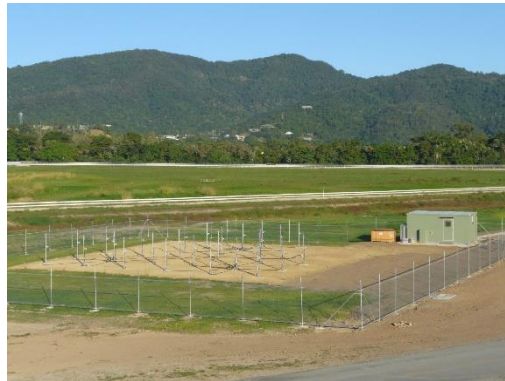
(Above) The Cairns BLP. The BLP system is a 12-kW peak power, 27 Yagi antenna array, three receive channel radar, which operates in SA mode. The antenna array covers an area of 16m x 16m. Data are provided by a 30-min BUFR data stream for weather forecasting and numerical weather model assimilation. Higher resolution (1-min) data are routinely produced for basic research purposes
