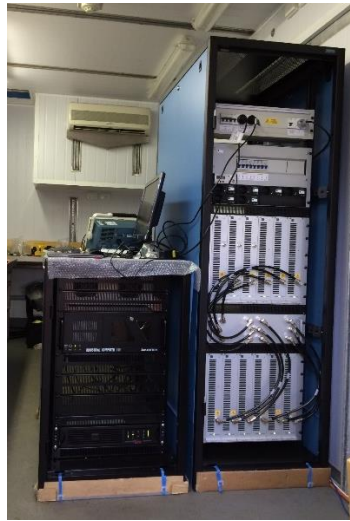
(Above) 40 kW EMDR radar with 6-channel digital transceiver. The power amplifier is the ATRAD 4 kW transmitter module. There are several hundred of these in operation. The receiving system is based on the ATRAD digital transceiver. There are several tens of these in operation.
