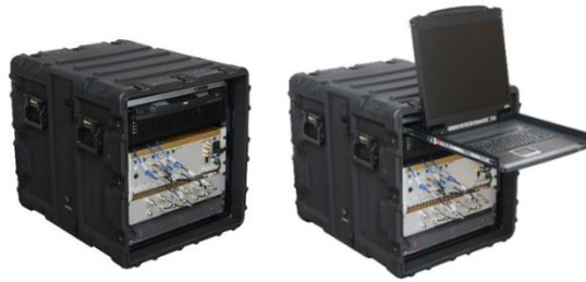
(Above left) The Remote Receiving system with keyboard and screen stowed, and (above right), with the keyboard and screen deployed. This figure shows the 6-channel transceiver, with Linux-PC, bandpass filter set and UPS.
