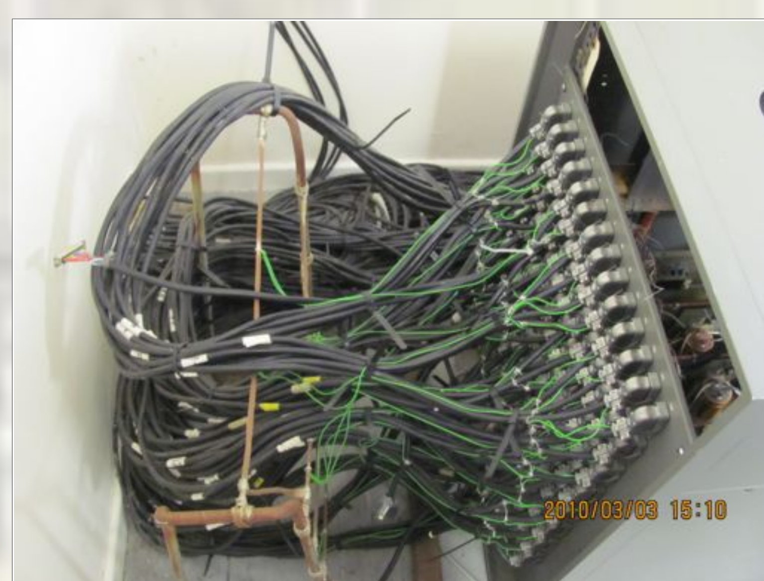
Fig5. Rear view of the original "Antenna Phasing Unit" showing the 100 interface cables to the Phase Shifters.
