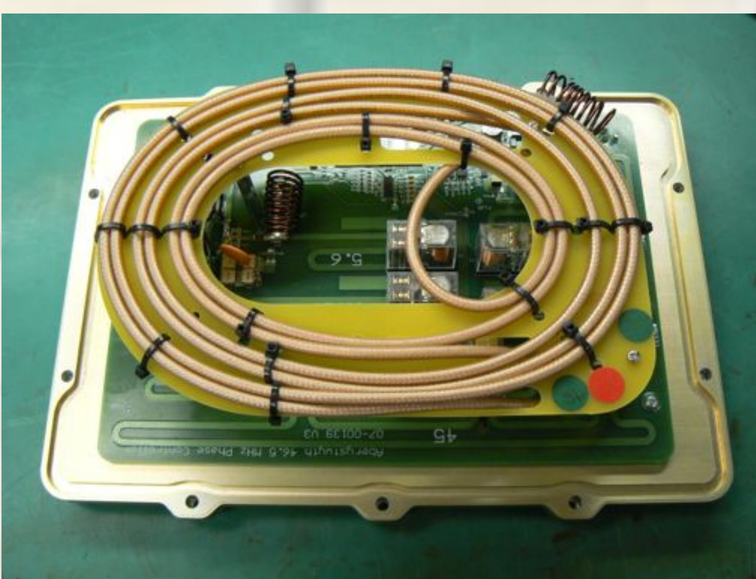
Fig 8. Internals of the new Phase Shifter unit.
