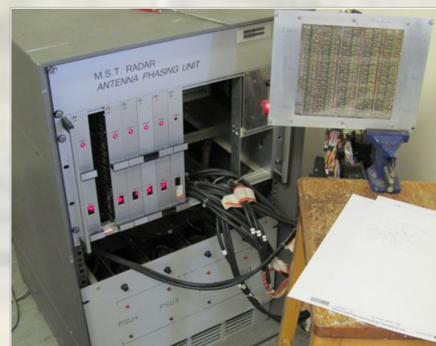
Fig4. Front view of the original "Antenna Phasing Unit" and Status Display
