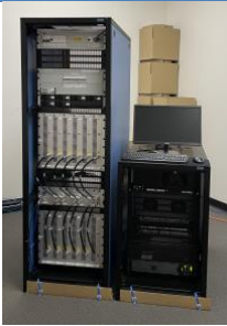
(Above) A six receiver channel 48 kW SII ionospheric radar. The radar power is expandable in 24 kW increments, and the receiver numbers in three channel increments
