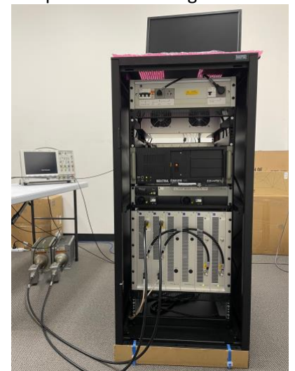
(Above) HF Broadband System undergoing Factory Acceptance Testing
