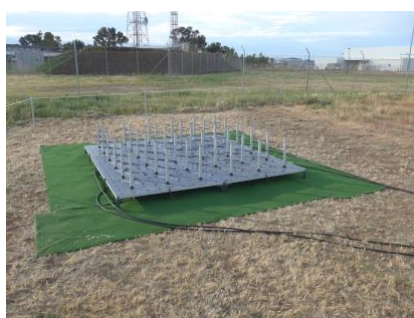
(Above) The 36-element UHF Yagi antenna array installed at Adelaide Airport. A Fabry Perot version is under development
